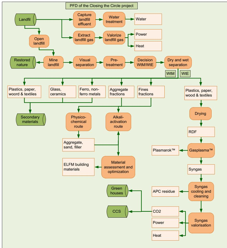
Fig. 6. General ELM process flow diagram for the Closing the Circle project (RDF = SRF = Solid Recovered Fuel).
