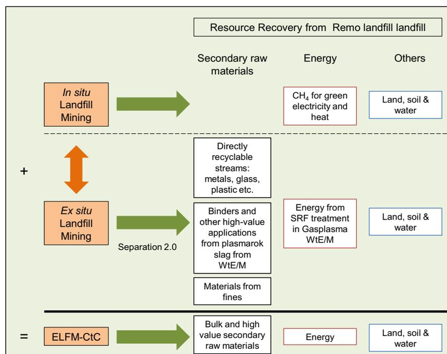
**Fig. 2.** Resource recovery from *in situ* and *ex situ* landfill mining – the double arrow indicates that for the Closing the Circle (CtC) project an *in situ* LFM phase (on landfill cells that are not excavated yet) can be combined with *ex situ* LFM (on landfill cells that are excavated).
