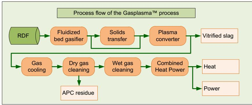
Fig. 5. Overview of the Gasplasma™ WtE/M process (RDF = Refuse Derived Fuel = SRF = Solid Recovered Fuel, Vitrified slag = plasmarok, APC = air pollution control).
