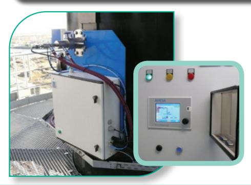
The AMESA is fast becoming the system of choice for new build energy from waste plants for the continuous sampling of dioxins and furans as standard.
