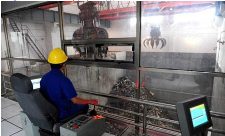
A Chinese worker controls robotic arms to throw rubbish into an incinerator at a plant in Qionghai, Southern Hainan province of China. Photograph: Corbis
