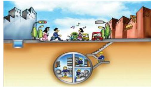
A common utility duct, sometimes called a common utility conduit, is any structure – above, on, or below ground – that carries more than two types of public utility lines.
